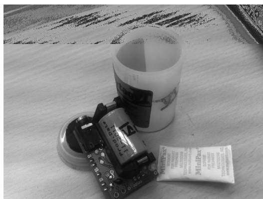
Fig.: 1: Tiny tag VI data logger with the 35mm film canister and packet with desiccant (Photo: T. Schaer).
